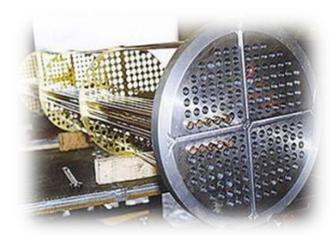
Units completely re-tubed to original specification or higher, tube plates baffles and shell also replaced when required. Work can be undertaken in our works, onsite or on board vessel to meet your requirements
