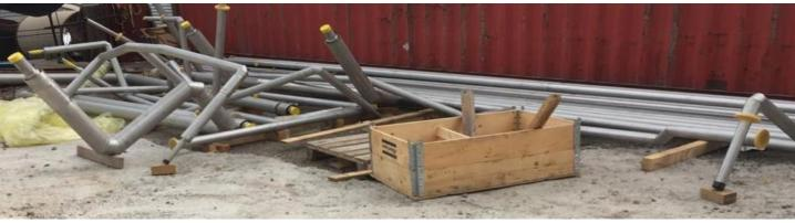
Vaccum piping has Approx, 256 no. of spools (13000 IM) and 5000 inch dia with a 1.5 to 4 mm thk. And 400 jhonstone coupling.
